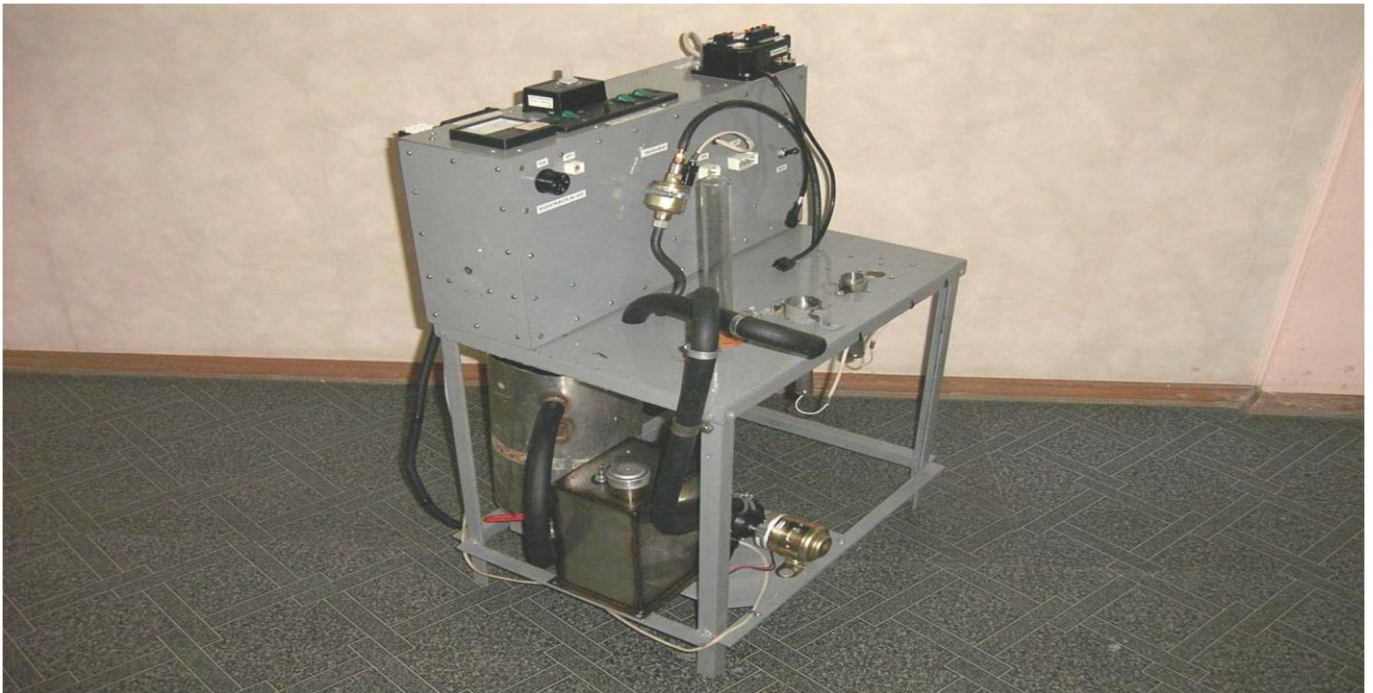
Fig. 13. Pre-heater test bench
